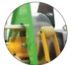
Heavy duty 3T decoiler with pneumatic snubber arm for improve safety.
