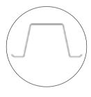
Web Roof batten: 15/8 x 37/16". Ceiling batten:  $\frac{7}{8} \times 2^{3}/8$ ". Gauge range from 26 - 22 gauge (16-27 mils).
