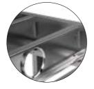
Accurate production of steel floor joists, pre-punched fixing tabs and service holes.
