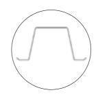
Web Roof batten: 40x87.5mm (1.57x3.45") Ceiling batten: 22-61mm (0.87x2.4"). Gauge range from 0.4mm to 0.8 mm (26 -22 gauge).
